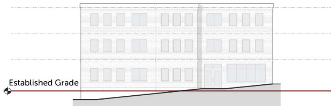
Figure 18: Section 11 – Established Grade (view from Front Lot Line)
